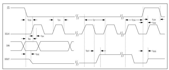
Figure 1. Detailed Serial-Interface Timing Diagram
