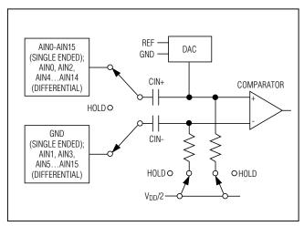
Figure 3. Equivalent Input Circuit
