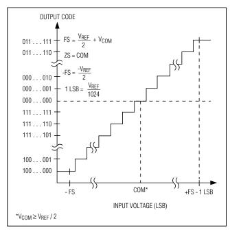
Figure 9. Bipolar Transfer Function, Full Scale ( $\pm FS$ ) =  $\pm V_{RFF}/2$
